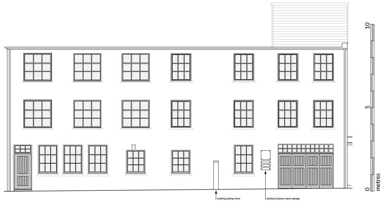
2 Existing East Elevation 1:50 @ A1
